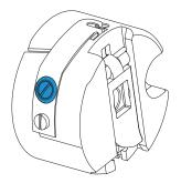
7. Once the thread tension in the bobbin case is correct, place the bobbin case inside the quilting machine with the **lever** (shown in blue) at the 3 o'clock position. It should click into place. Do not pull on the lever while inserting the bobbin case.
